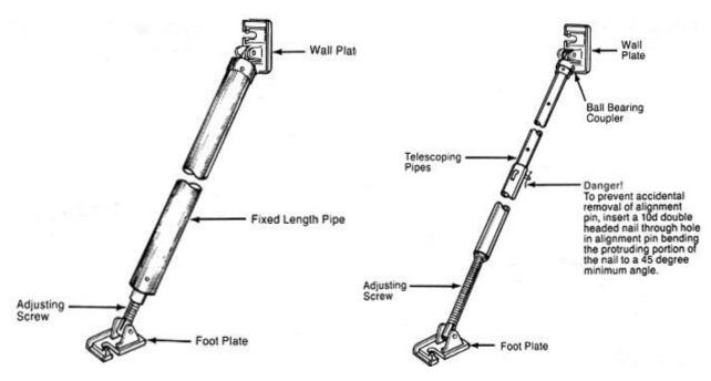
To fix the brace to the footing or panel bolts or nuts with washers of the correct grade and size must be used. The anchor bolt and washer combination on the foot of the brace should have adequate bearing capacity. Sometimes the bolt head and washer are too small for the slot size on the brace foot. This can cause the washer to collapse and the panel to move. As a general principle the slot width on the brace foot should not
