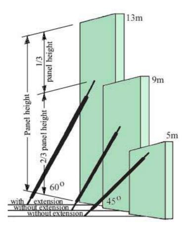
Bracing should be installed in accordance with AS 3850 and the approved shop drawings Braces are usually installed at an angle of 45° to 60° and square to the line of the panel Generally two (2) braces are used to support each panel Where a single brace is used (eg on narrow panels) to brace a panel particular care is required.
